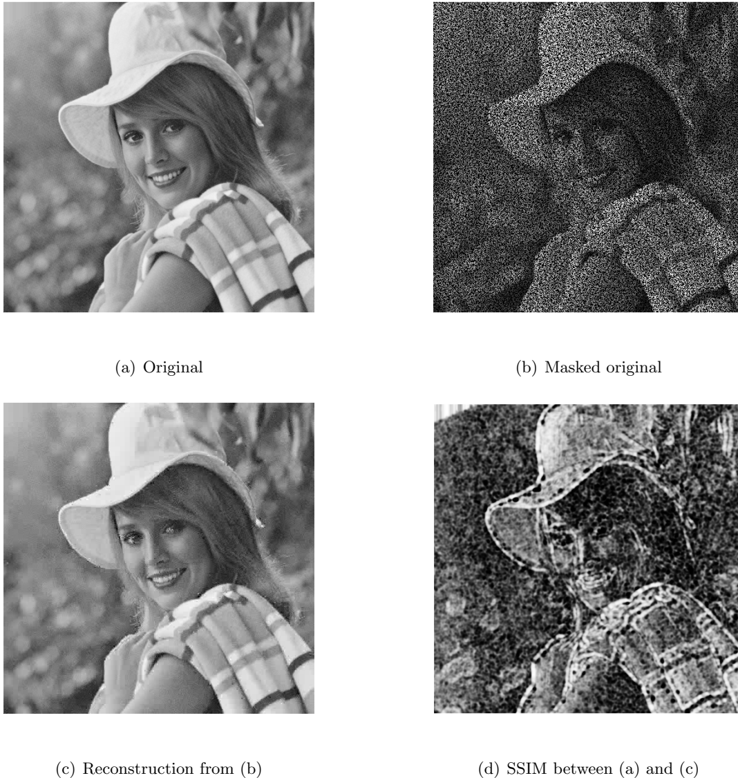
Figure 13: Reconstruction of image Elaine from a deterministic sampling mask with 50% density and \epsilon = 4\sqrt{32} . The reconstruction is achieved at 29.8081 dB and has an MSSIM equal to 0.7461.
