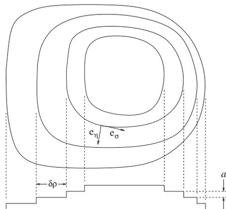
FIG. 1. Schematic of steps (top and side views). Local coordinates are  $(\eta, \sigma)$ ;  $\eta = \eta_i$  at the  $i$ th edge.
