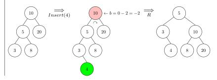
**Example 5.2.** An example of insertion resulting in a left-right heavy tree, fixed by a left-right rotation:
