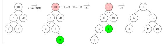
**Example 5.3.** Another example of insertion resulting in a left-left heavy tree, fixed by a right rotation:
