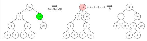
**Example 6.2.** An example of deletion resulting in a left-right heavy tree fixed by a left-right rotation:
