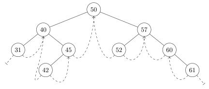
Observe that the node with key 31 has no inorder predecessor because it is the first key in the inorder traversal. Similarly the node with key 61 has no inorder successor because it is the last key in the inorder traversal.
