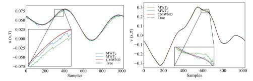
Figure 5: The output of GS couple equations at the initial condition (U-Rand, V-GRF). (Left) The predicted output of the models to  $u(x, \tau = 1)$ . (Right) The predicted output of the models to  $v(x, \tau = 1)$ .
