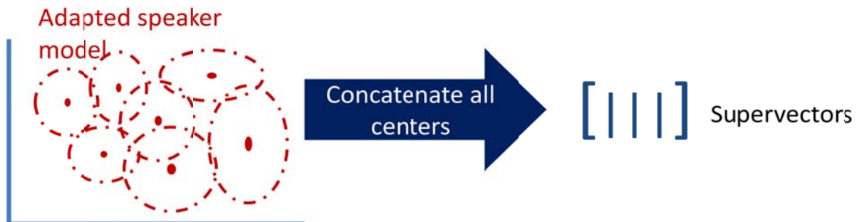
Figure 4: Creation of supervectors from GMMs (Courtesy of Balaji Srinivasan)
