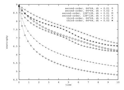
Figure 6.14: Enstrophy plot for the "thick" shear-layer problem
