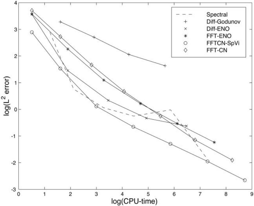
FIG. 2.  $L^2$  error vs CPU-time.
