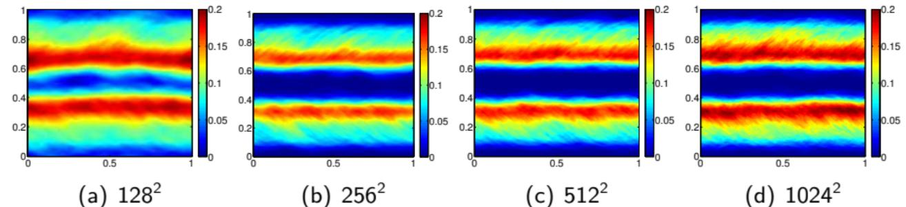
**Figure:** Approximate sample variances of the density for the Kelvin-Helmholtz problem at  $t = 2$  and different mesh resolutions. All results are with 400 Monte Carlo samples.
