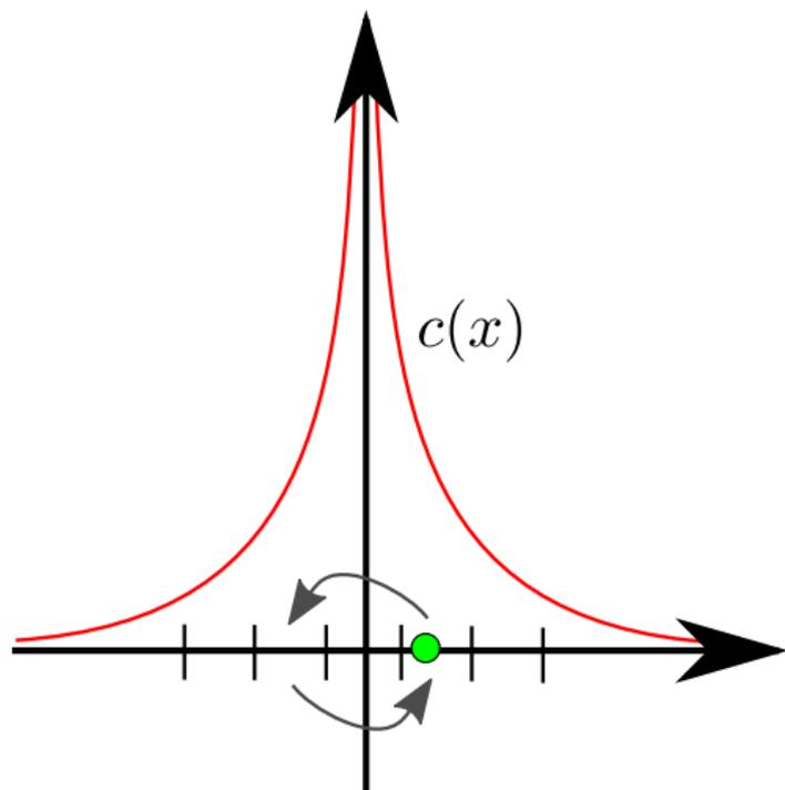
To avoid oscillations, choose  $\Delta\tau^{(i)}$  such that particle can only jump into adjacent cell  $\Delta t = \Delta\tau^{(1)} + \dots + \Delta\tau^{(k)}$
