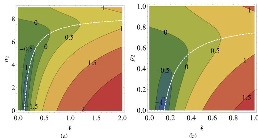
Figure 3: Contour plot of  $\log[r_a]$  for  $N = 10$  agents coupled over (a) NC networks with  $n_1 = 8$ , and  $n_2$  and  $\hat{\epsilon}$  varying (b) Erdos-Renyi networks with  $p_1 = 0.8$ ,  $p_2$  and  $\hat{\epsilon}$  varying. The optimum value of  $n_2$ , and the optimum value of  $p_2$ , are denoted by the dashed white line.
