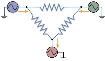
(simplified) **swing equation** model of interconnected synchronous generators:
