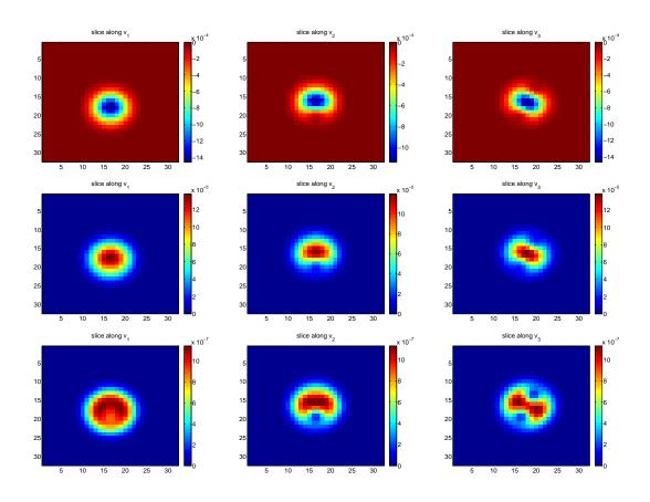
Figure 3:  $f^{\text{fast}} - f^{\text{direct}}$  at time t = 6. From left to right: slices along the direction of  $v_1$ ,  $v_2$  and  $v_3$ . From top to bottom:  $f^{\text{fast}}$  obtained with M = 14, 38 and 74. Other parameters are the same as in Figure 2.
