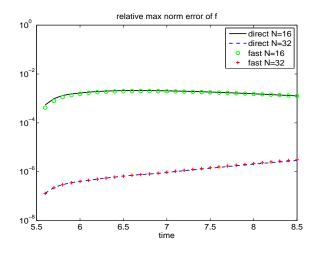
Figure 1: Time evolution of  $||f^{\text{num}} - f^{\text{ext}}||_{L^{\infty}}/||f^{\text{ext}}||_{L^{\infty}}$ . RK4 with  $\Delta t = 0.1$  for time discretization. Other parameters are the same as in Table 1.
