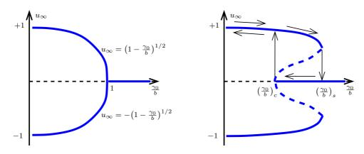
FIG. 4.1. Left: pitchfork bifurcation diagram for the stationary equilibrium solution  $u_{\infty}$  for  $\alpha=2$ . Right: sub-critical pitchfork bifurcation diagram for the stationary equilibrium solution  $u_{\infty}$  for  $\alpha>6$ . The arrows highlight the hysteresis loop.
