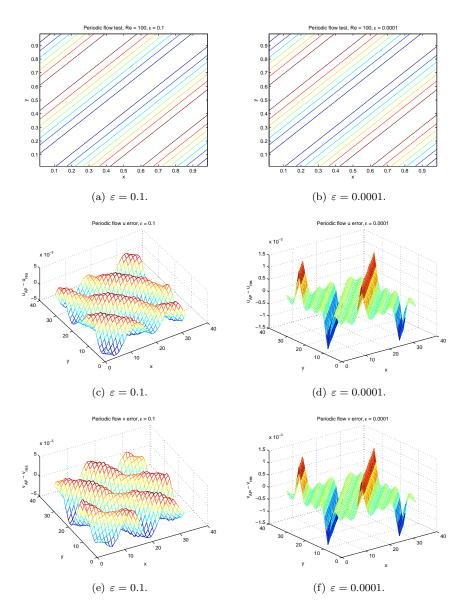
Figure 4: Results for periodic flow test case (38). Left column:  $\varepsilon = 0.1$ . Right column:  $\varepsilon = 10^{-4}$ . Top row: stream function of solution with  $\Delta x = 1/16$ . Middle row: error in u. Bottom row: error in v
