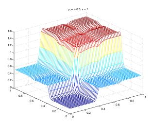
Figure 3: Density plot of 2D Riemann problem with initial data (37).  $\varepsilon = 1, \gamma = 1.4, \alpha = 0.5$ .
