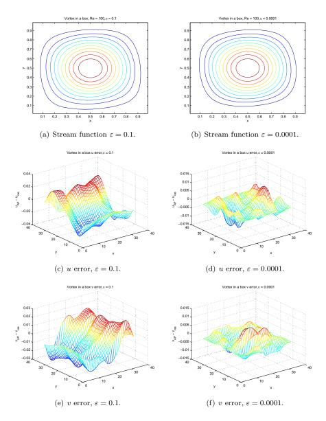
Figure 5: Results for vortex in a box flow (39) at T = 0.125. Left column:  $\varepsilon = 0.1$ . Right column:  $\varepsilon = 10^{-4}$ . Top row: stream function of solution with  $\Delta x = 1/16$ . Middle row: error in u. Bottom row: error in v
