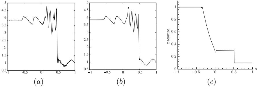
FIGURE 3.11. Computations using the Legendre spectral viscosity scheme (3.28). (a) A density field in Euler equations, (2.7a), using  $N = 220$  modes. (b) The density field after postprocessing. (c) the pressure field after postprocessing (compare with the FEM solution in Figure 3.6(b)).
