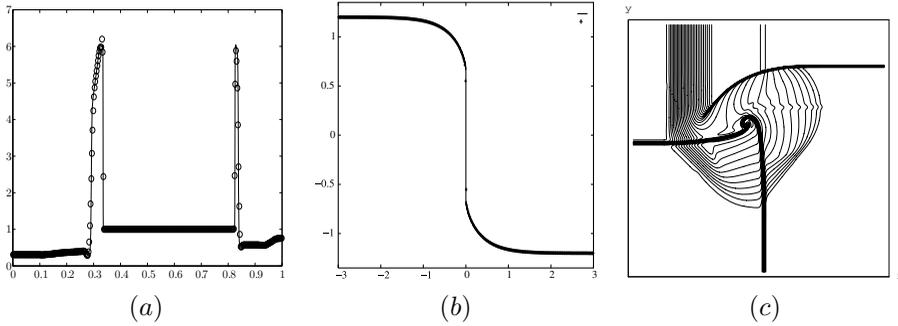
FIGURE 3.8. Numerical solution using FV central schemes. (a) Density of compressible Euler equations computed at  $t = 0.01$  using a central discontinuous Galerkin method [142]. (b) Saturating dissipation,  $w_t + f(w)_x = (w_x / \sqrt{1 + w_x^2})_x$  [126]. (c) Density contours of two-dimensional Riemann problem (without a Riemann solver).
