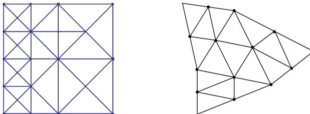
FIGURE 3.5. Structured and unstructured triangulation of two-dimensional domains.
