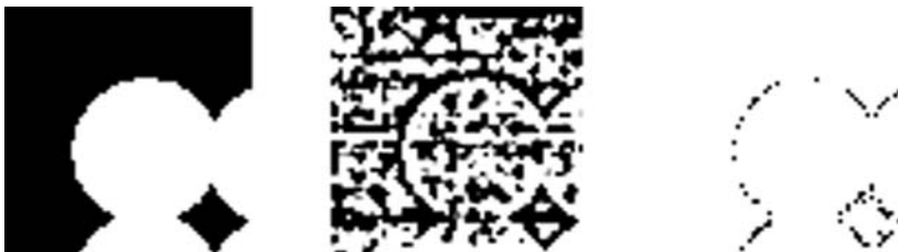
Fig. 7 Demonstrating the recovery results by zero crossing compressed sensing model. The available 2000 data points are uniformly and randomly distributed over 64^2 grids. Left: original image. Center: the image recovered from incomplete data by back projection method. Right: the result obtained by zero crossing compressed sensing method. Here we choose the parameters \gamma = 3
