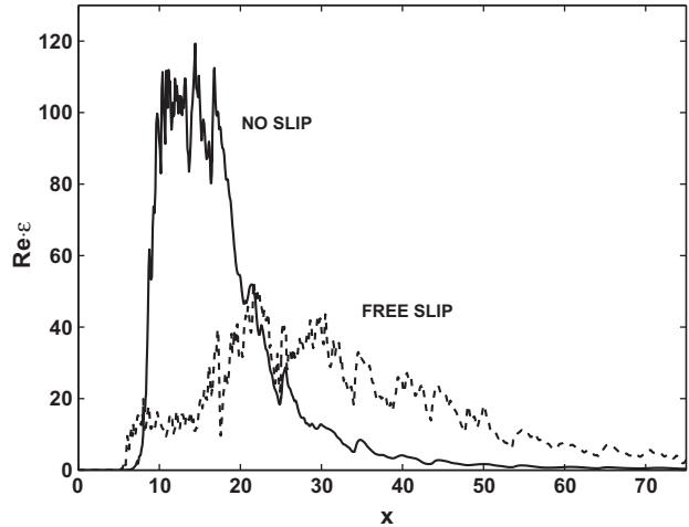
**Fig. 15.** Dissipation rate of turbulent kinetic energy  $\varepsilon$  times  $Re$  versus streamwise  $x$ -direction  $y = z = 0$  for  $h = 1$ . The continuous line depicts NS conditions and the dashed one FS conditions.
