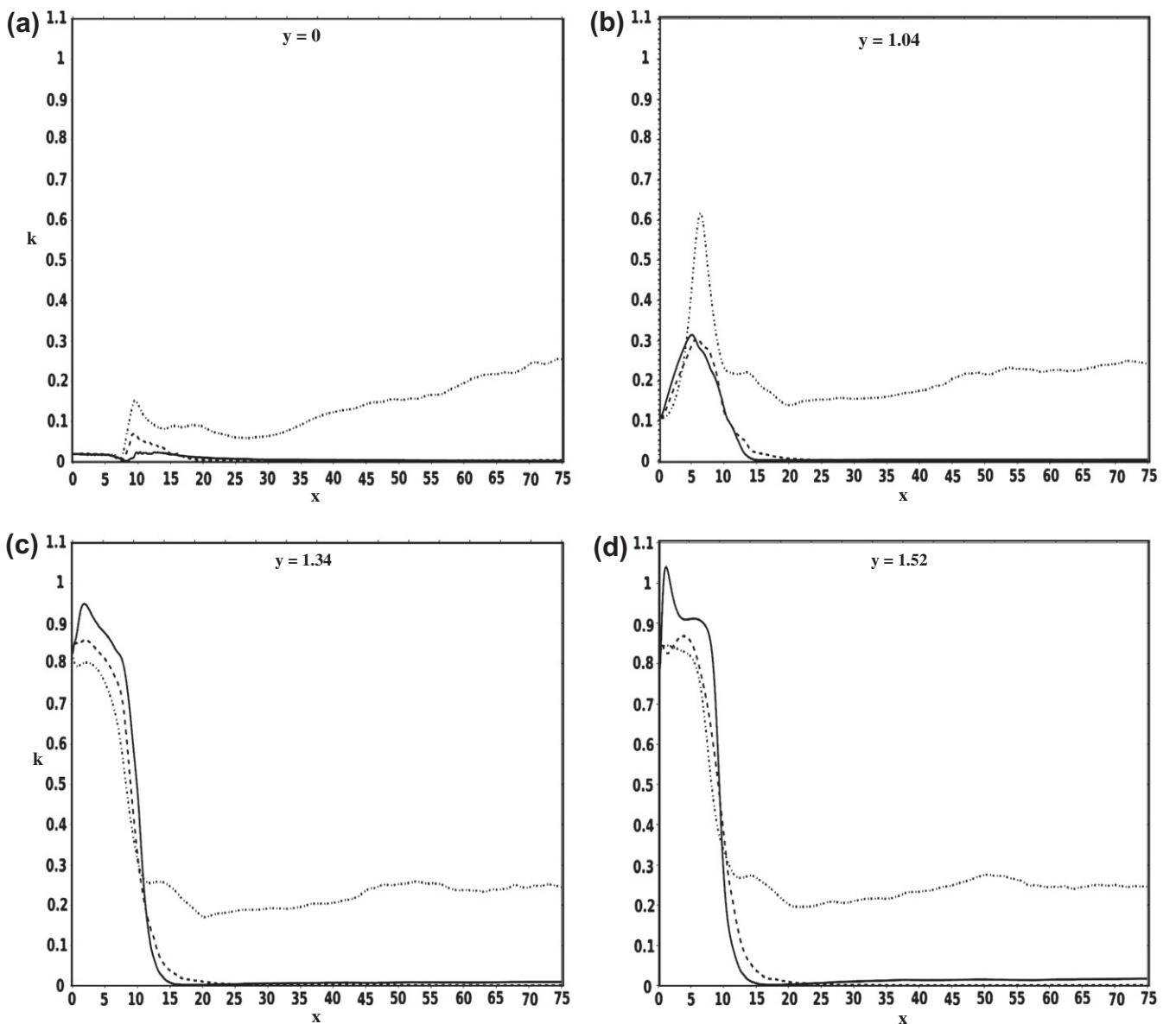
**Fig. 10.** Turbulent kinetic energy  $k$  versus streamwise  $x$ -direction for  $h = 3$  (dotted line),  $h = 1$  (dashed line) and  $h = 0.7$  (solid line), at (a)  $y = 0$ , (b)  $y = 1.04$ , (c)  $y = 1.34$  and (d)  $y = 1.52$ .
