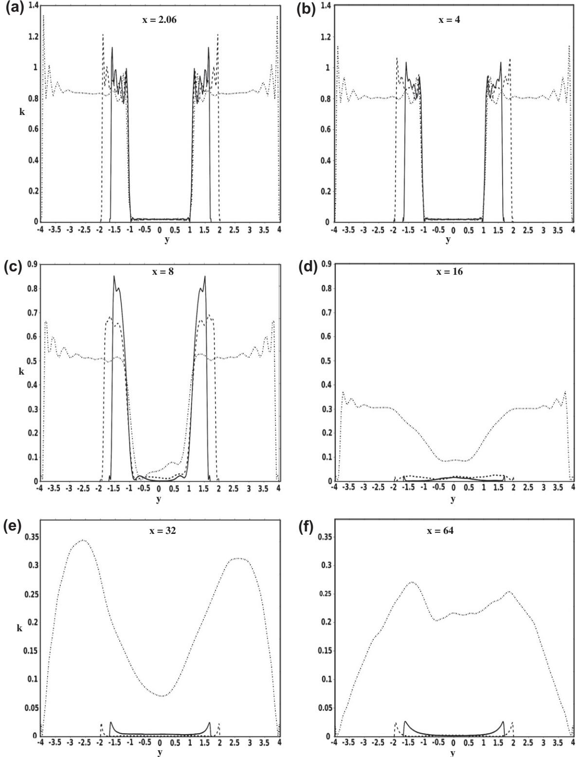
**Fig. 9.** Turbulent kinetic energy  $k$  versus crossflow  $y$ -direction for  $h = 3$  (dotted line),  $h = 1$  (dashed line) and  $h = 0.7$  (solid line), at (a)  $x = 2.04$ , (b)  $x = 4$ , (c)  $x = 8$ , (d)  $x = 16$ , (e)  $x = 32$  and (f)  $x = 64$ .
