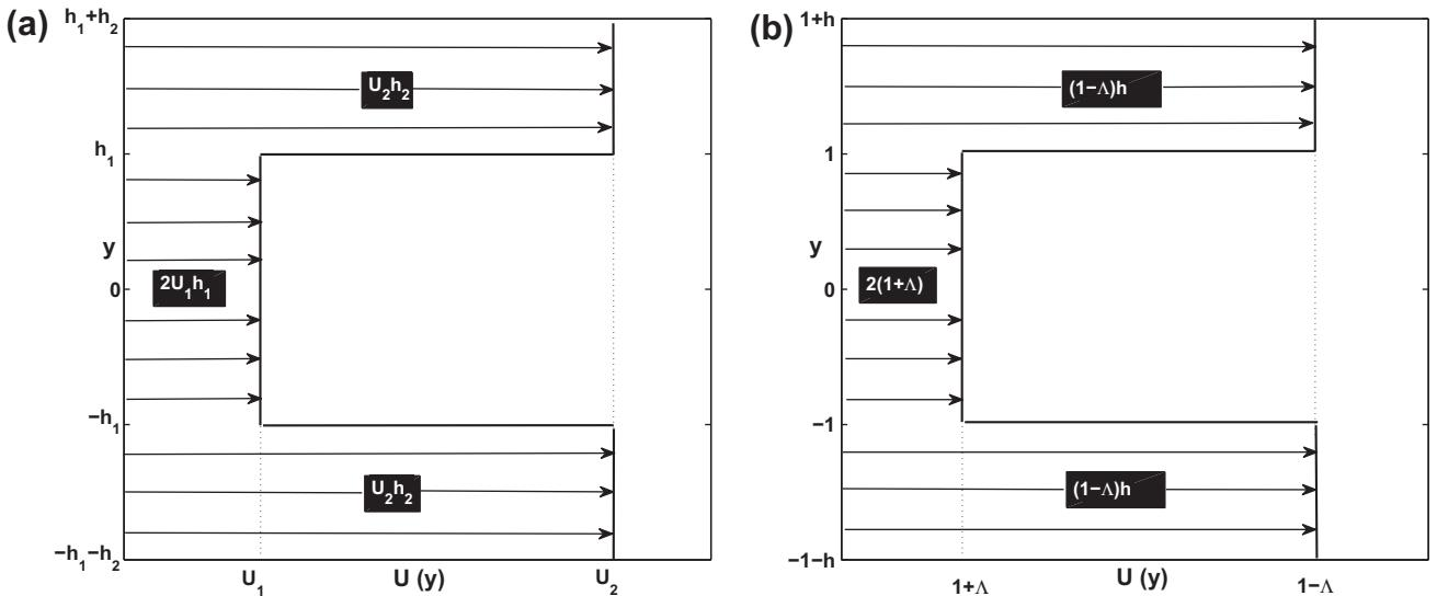
**Fig. 1.** Schemas of the inlet velocity profile, using dimensioned values (a) and dimensionless values (b). The black squares indicate the flowrates (per unit thickness) that correspond to each part of the flow.
