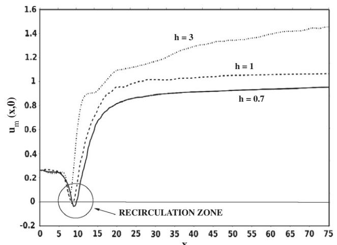
**Fig. 8.** Mean streamwise velocity  $u_m(x, 0)$  versus the streamwise  $x$ -direction for  $h = 3$  (dotted line),  $h = 1$  (dashed line) and  $h = 0.7$  (solid line). A recirculation region is only present for  $h = 0.7$  and  $h = 1$ .
