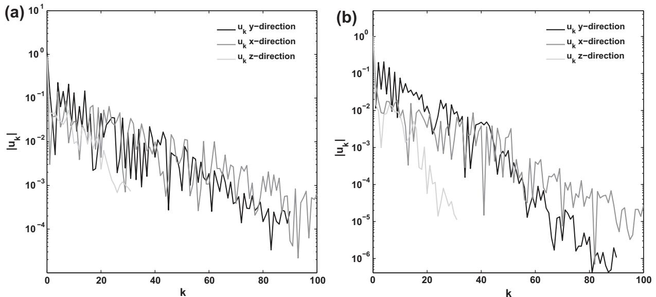
Fig. 2. Chebyshev spectra and modulus of the Fourier spectrum of the streamwise velocity as computed, for  $h = 1$ , from the  $x$ ,  $y$  and  $z$ -axis issued from the points (23.58, 0, 0) (a) and (51.58, 0, 0) (b).
