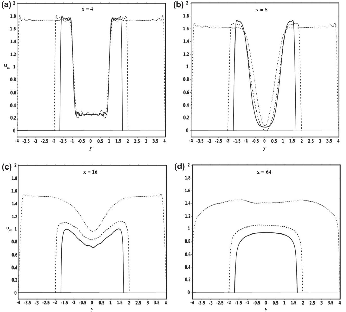
**Fig. 7.** Mean streamwise velocity profile  $u_m(x, y)$  versus the crossflow direction  $y$  for  $h = 3$  (dotted line),  $h = 1$  (dashed line) and  $h = 0.7$  (solid line), at different abscissa: (a)  $x = 4$ , (b)  $x = 8$ , (c)  $x = 16$  and (d)  $x = 64$ .
