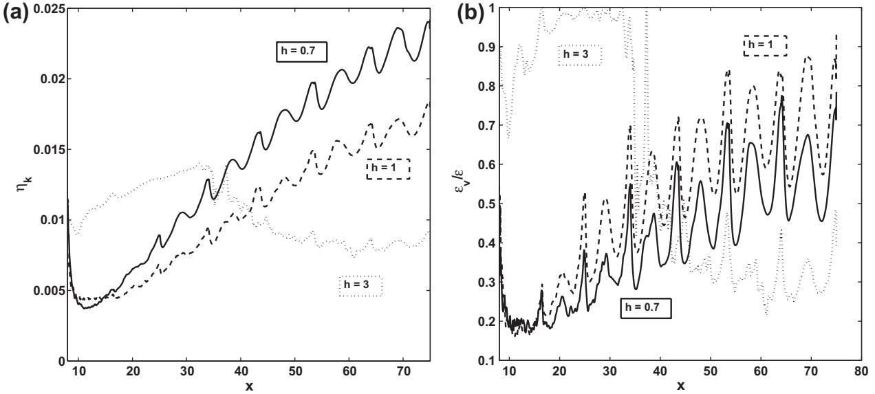
**Fig. 12.** (a) Kolmogorov scale and (b) ratio between physical and total dissipation rates versus streamwise  $x$ -direction  $y = z = 0$ , for  $h = 3$  (dotted line),  $h = 1$  (dashed line) and  $h = 0.7$  (solid line).
