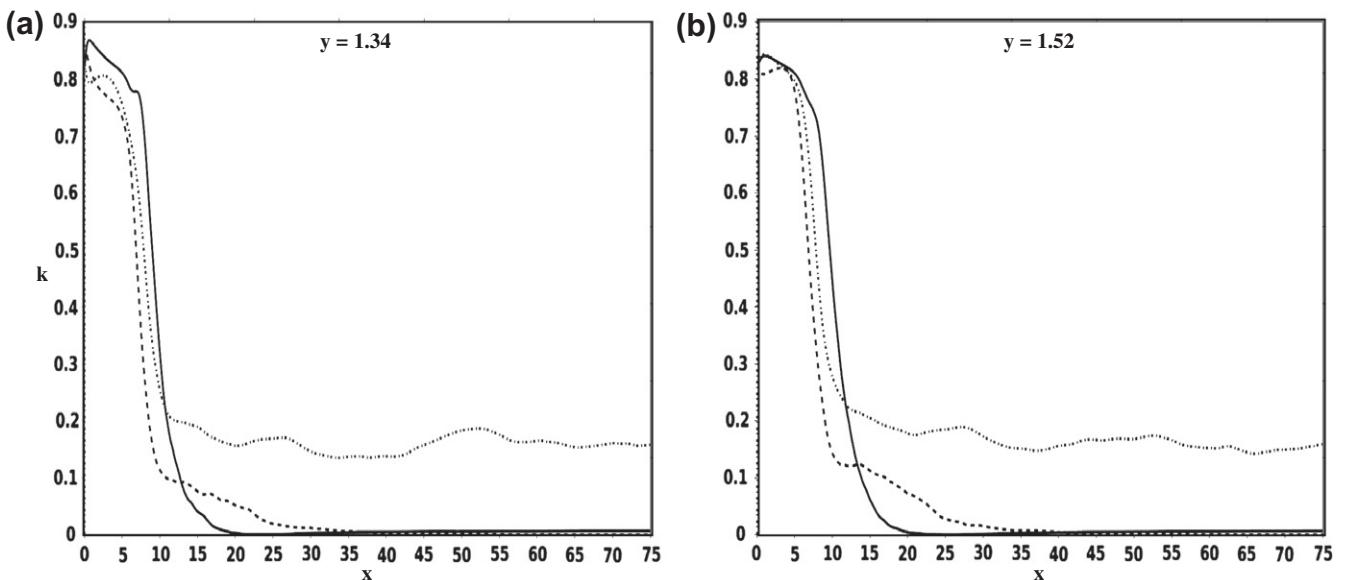
**Fig. 14.** Turbulent kinetic energy for the FS-flows with respect to streamwise direction  $x$  at (a)  $y = 1.34$  and (b)  $y = 1.52$ , for  $h = 3$  (dotted line),  $h = 1$  (dashed line) and  $h = 0.7$  (solid line).
