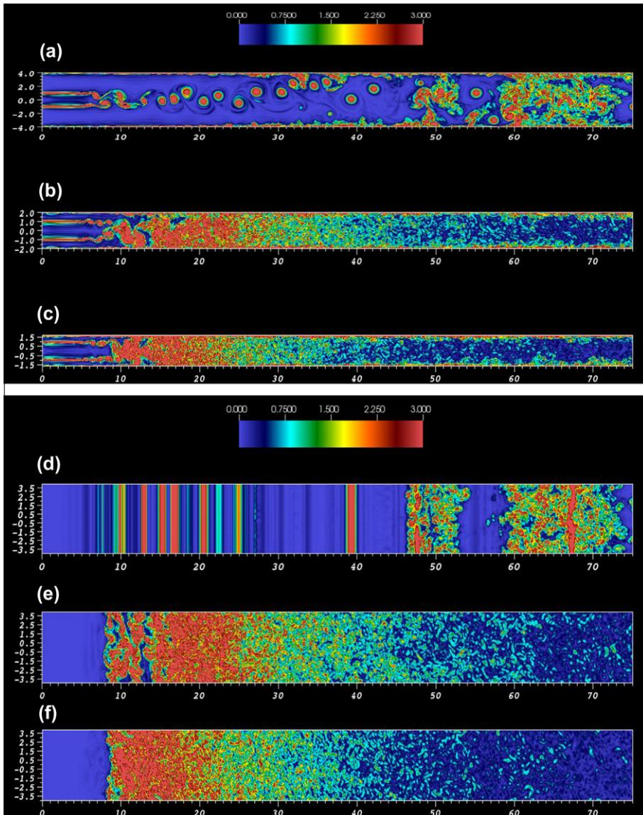
**Fig. 3.** Instantaneous modulus of the vorticity  $|\omega|$  in the central planes  $z = 0$  (top) and  $y = 0$  (bottom) at  $t = 400$  for (a, d)  $h = 3$ , (b, e)  $h = 1$  and (c, f)  $h = 0.7$ ;  $Re = 5000$ .
