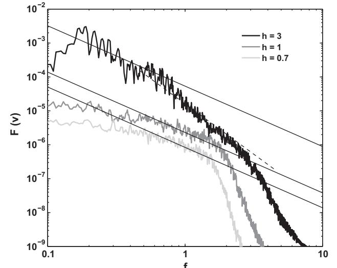
**Fig. 5.** Fourier spectra of the velocity crossflow component  $v(x = 51.85, y = 0)$ , for  $h = 3$  (black line),  $h = 1$  (dark gray) and  $h = 0.7$  (light gray). Thin lines represent the slopes  $-5/3$  (continuous) and  $-3$  (dashed).
