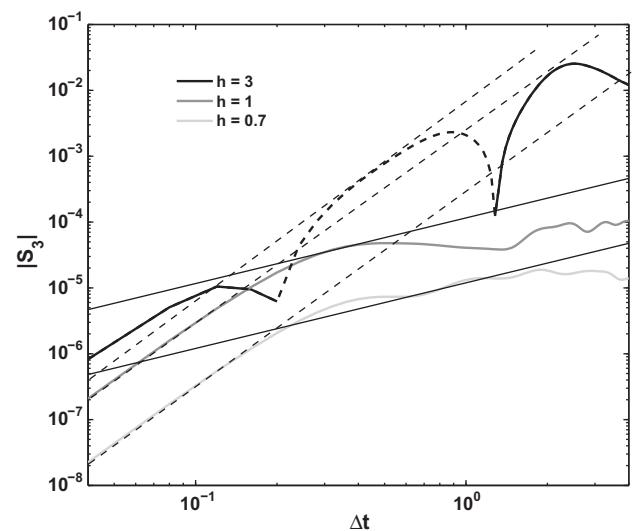
**Fig. 6.** Absolute value of the third order structure function  $S_3$  versus time shift  $\Delta t$  for  $v(x = 51.85, y = 0)$ , for  $h = 3$  (black line),  $h = 1$  (dark gray) and  $h = 0.7$  (light gray). Continuous lines depict negative values of  $S_3$  and dashed lines depict positive values. Thin lines represent the slopes 1 (continuous) and 3 (dashed).
