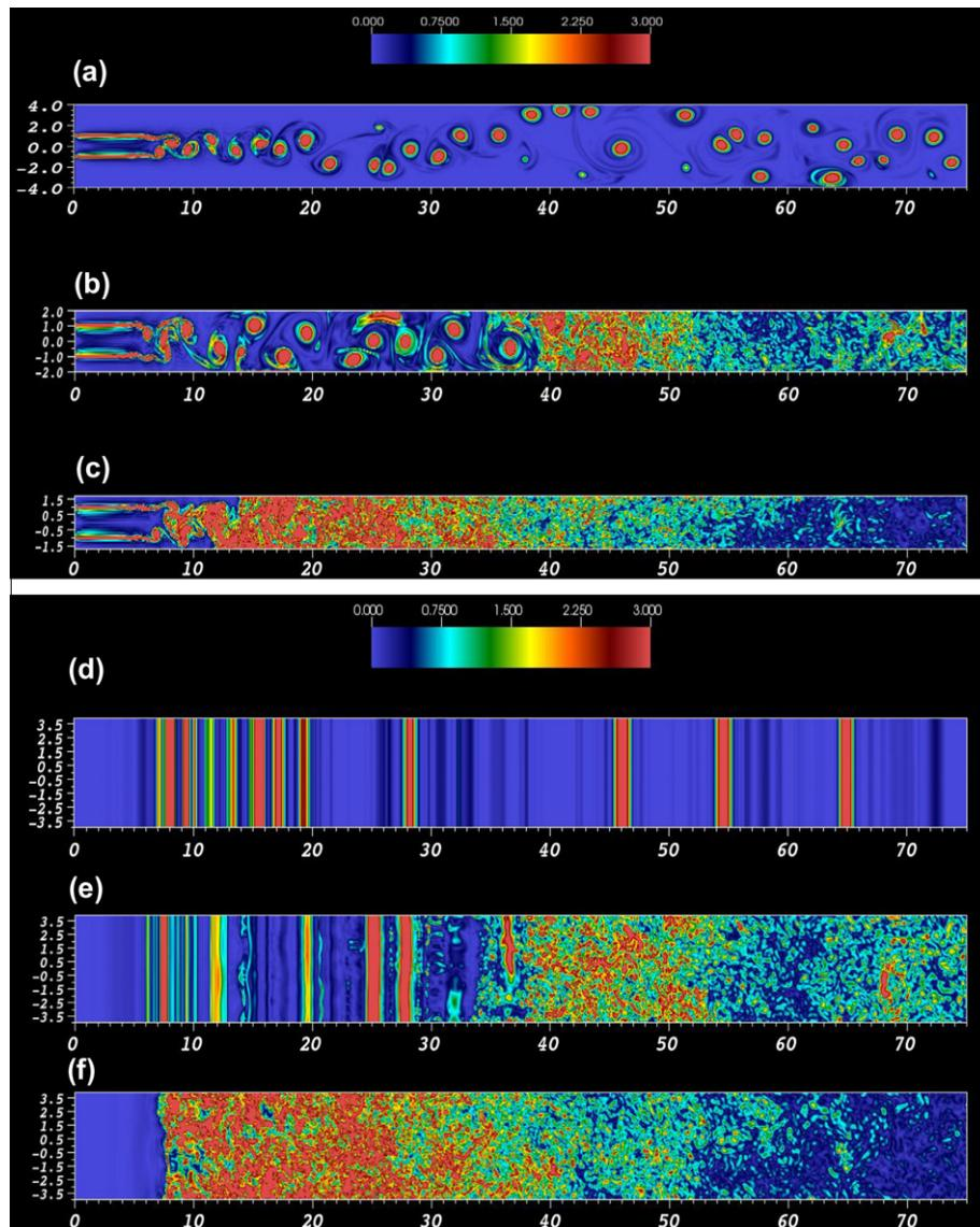
Fig. 13. Instantaneous modulus of the vorticity  $|\omega|$  in the central planes  $z = 0$  (top) and  $y = 0$  (bottom) at  $t = 400$  for FS-flows: (a, d)  $h = 3$ , (b, e)  $h = 1$  and (c, f)  $h = 0.7$ .
