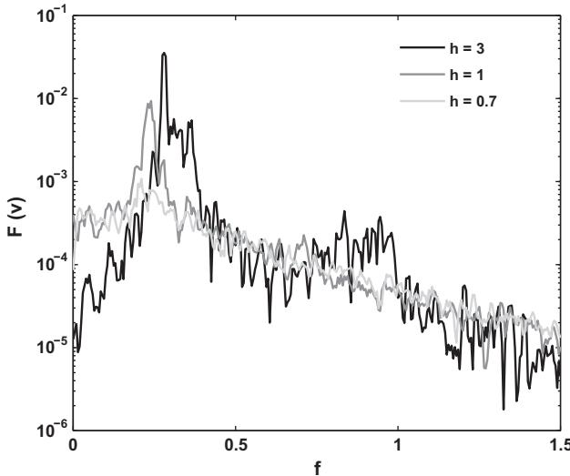
**Fig. 4.** Fourier spectra of the velocity crossflow component  $v(x = 12.25, y = 0)$ , for  $h = 3$  (black line),  $h = 1$  (dark gray) and  $h = 0.7$  (light gray). The dominant frequency is decreasing with confinement.
