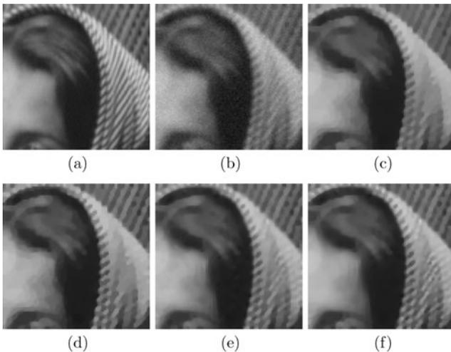
**Fig. 14** *Example 3:* Results of different methods when restoring the blurred and noisy image “Barbara”: (a) Original image, (b) Blurred noisy image, (c) TV-method (PSNR = 28.06, MSSIM = 0.823), (d) Bregman iteration (PSNR = 28.27, MSSIM = 0.839,  $k = 76$ ), (e) TNV-method (PSNR = 29.15, MSSIM = 0.865,  $k = 9$ ), (f) Our method (PSNR = 29.68, MSSIM = 0.883,  $k = 4$ )
