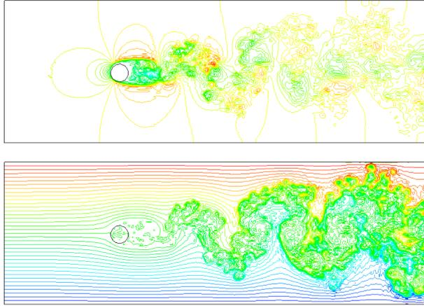
FIG. 1: Streamwise velocity (top) and temperature (bottom) instantaneous fields in the median vertical plane,  $Re = 3900$ ,  $F = 75$ ,  $Pr = 7$ .
