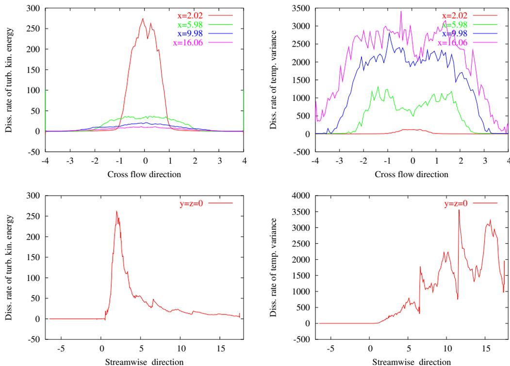
FIG. 3: Dissipation rates of the turbulent kinetic energy times  $Re$  (left) and temperature variance times  $Pe$  (right) at different  $x$ -locations (top) and along the streamwise central line (bottom).
