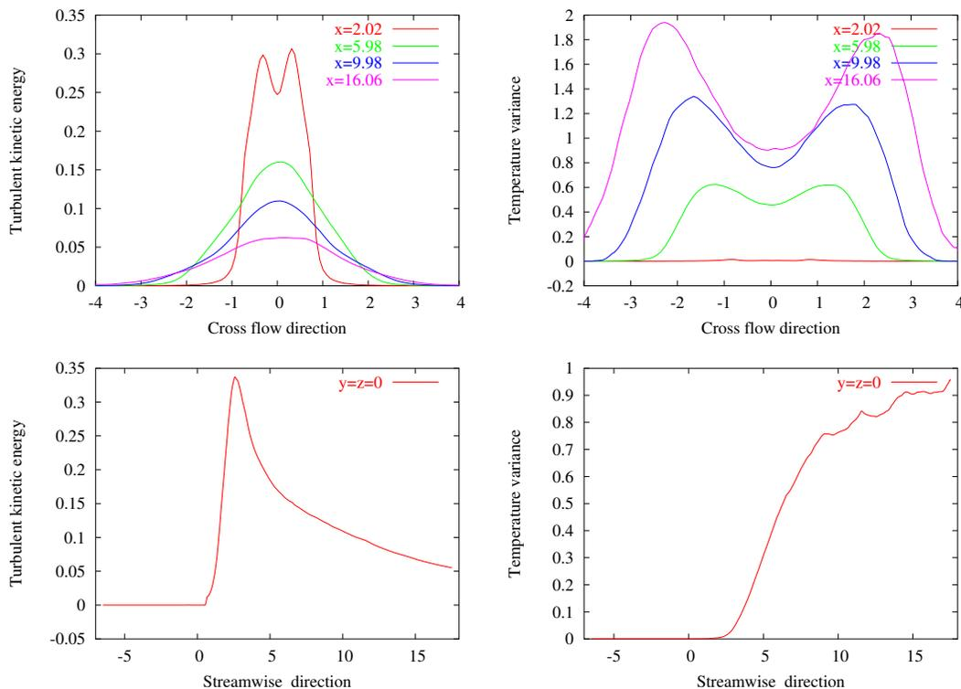
FIG. 2: Turbulent kinetic energy (left) and temperature variance (right) at different  $x$ -locations (top) and along the streamwise central line (bottom).
