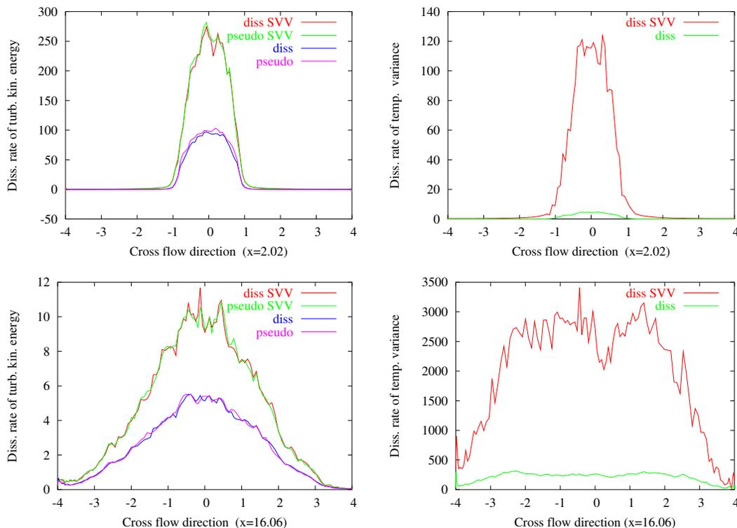
FIG. 4: Dissipation and pseudo-dissipation rates of the turbulent kinetic energy times  $Re$  (left) and dissipation rate of the temperature variance times  $Pe$  (right) from the SVV modified and standard formulations of these rates at two  $x$ -locations.
