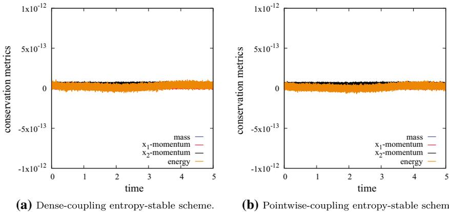
**Fig. 4** Two-dimensional isentropic vortex test case. Conservation of mass, momentum, and energy on a coarse non-conforming curved grid
