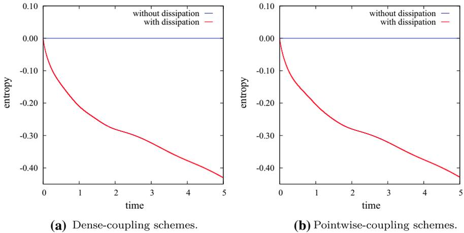
**Fig. 5** Two-dimensional isentropic vortex test case. Conservation and dissipation of entropy on a coarse non-conforming curved grid
