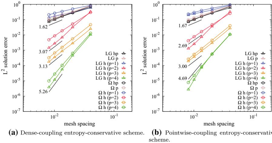
**Fig. 7** Two-dimensional isentropic vortex test case. Convergence studies of the entropy-conservative schemes on curved non-conforming grids (the convergence rates of the three finest grids are provided)
