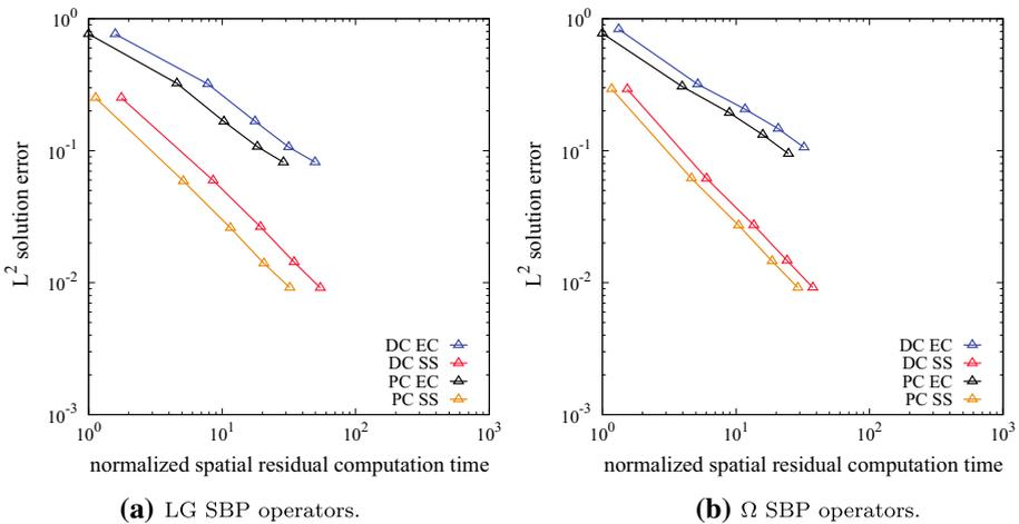
**Fig. 9** Two-dimensional isentropic vortex test case. Efficiency study of the entropy-conservative and entropy-stable schemes on curved non-conforming grids
