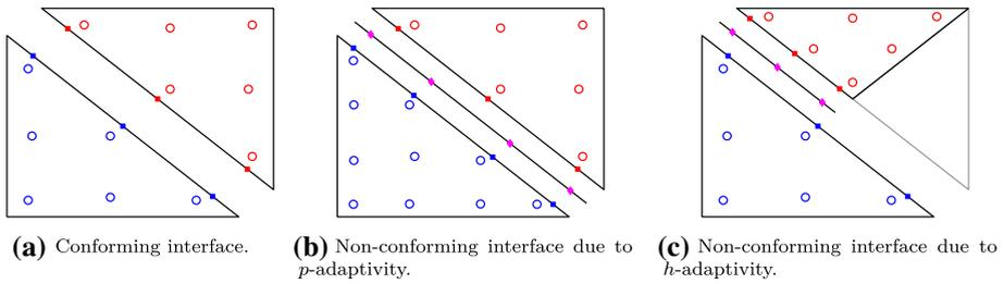
**Fig. 2** Visualization of coupling of conforming and non-conforming neighbouring elements. Non-conforming elements require an intermediate interface
