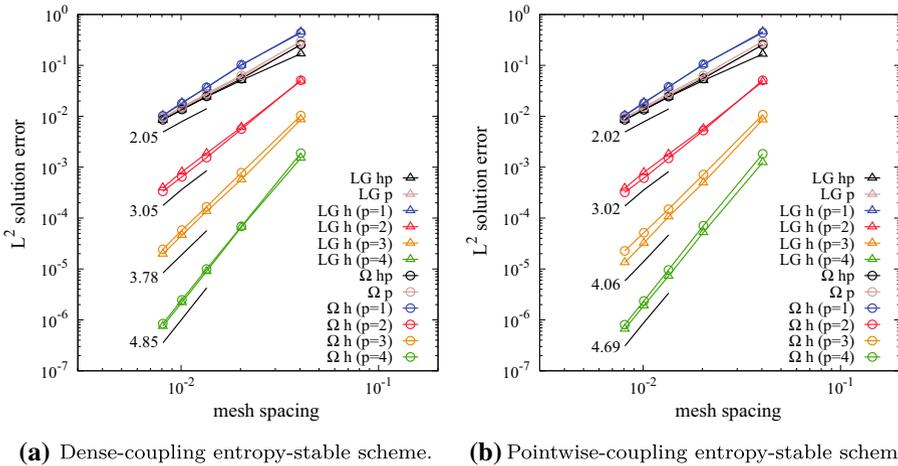
**Fig. 8** Two-dimensional isentropic vortex test case. Convergence studies of the entropy-stable schemes on curved non-conforming grids (the convergence rates of the three finest grids are provided)
