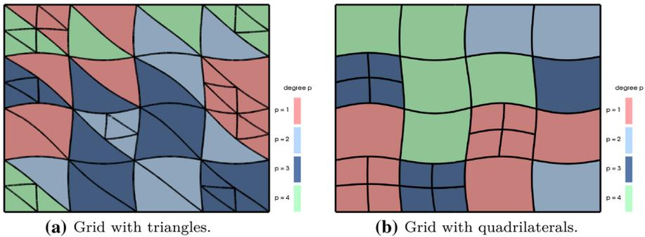
**Fig. 3** Two examples of coarse non-conforming curved grids with hanging nodes and different degree operators
