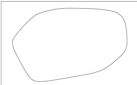
FIGURE 13.4. A piecewise conic
